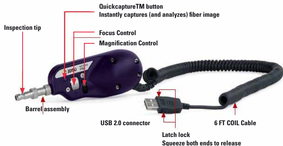
Fig. 16 Probe components
