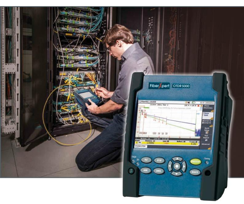
Designed with the installers and operators of enterprise networks in mind, the FiberXpert OTDR 5000 measures, documents and troubleshoots fiber optic networks. The FiberXpert OTDR 5000 provides very high resolution with one of the shortest dead zones available for testing multimode and single-mode fibers, thus enabling measurement of very short fiber links. Automatic analysis features simplify the measurement tasks
