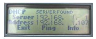
PINGER PLUS+ displays the responding IP Address of the DHCP Server and the IP Address assigned to the PINGER PLUS+.
