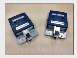
Test your CAT6A patch cords in 9 sec from both ends, and test twice as many patch cords per replaceable jack
