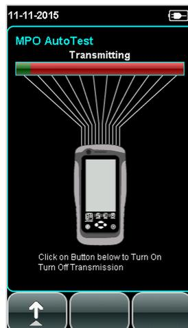
3. Press the AUTOTEST button on the Local unit to begin test.
