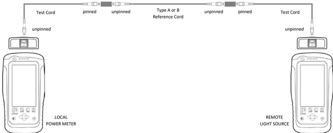
4. Press the [TOOLS] button → **Set Reference** and press the [Ok] button to set reference.
